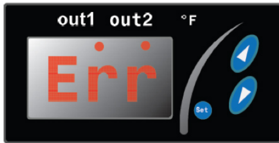
Figure 3 - Digital Temperature Controller Error Display
